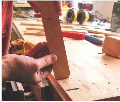
▲ Pic.2 ...ready for the tenons on the front rails
